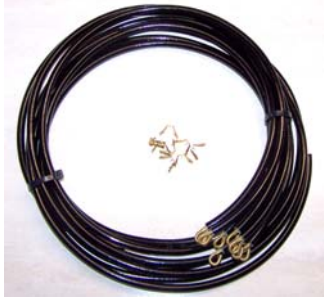
SPW-101 1932-36 FORD SPARK PLUG WIRE SET V-8 7MM BLACK LACQUERED WIRE CRIMPED ON BRASS HOOKED TERMINALS 8 BRASS DISTRIBUTOR CLIPS $55.00
