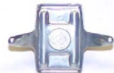
2478 10-24 X 1/2" BOLT 1952-56 FORD, MERCURY REAR DOOR, QUARTER PANEL, REAR WINDOW MOULDING CLIP $1.50
