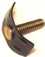
2673 '57 FORD 10-24 X 3/4" STUD QUARTER PANEL MOULDING CLIP (B7A5825562-A) $1.50
