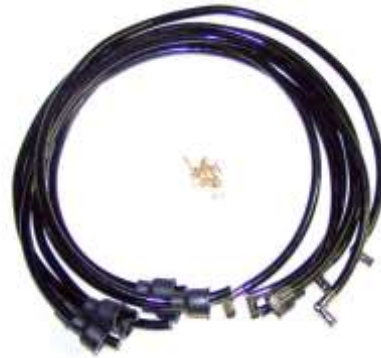
WS-111 1929-54 DODGE 6CYL SPARK PLUG WIRE SET 7MM BLACK LACQUER WIRE CORRECT 90° ANGLED ENDS $30.00
