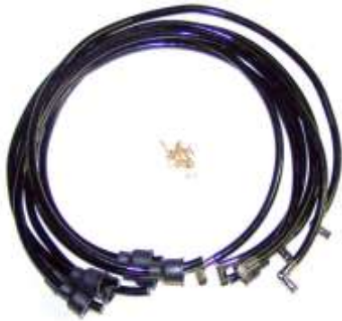
WS-130 1929-54 PLYMOUTH 6CYL SPARK PLUG WIRE SET 7MM BLACK LACQUER WIRE CORRECT 90° ANGLED ENDS $30.00
